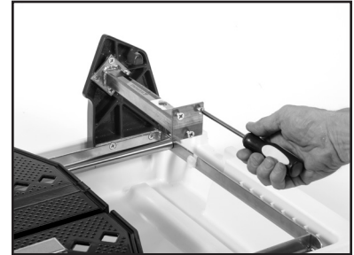
(C) Locate and remove the three Cutting Head Retaining Screws using a Phillips Screwdriver.
