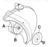
Lock the shaft. Insert a tool in the hole in the cutting head and rotate the blade until it is locked.
