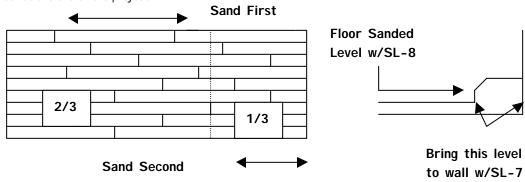
Use the SL-8 sander for the main section of the floor and then follow with the SL-7 edger. This method will allow you to set the level you want in the main section of the floor and than bring it out to the edge of the room with the SL-7.
