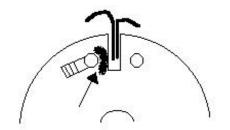
Insert 20 grit paper, move cam back so the spring pressure is not on the sawdust
