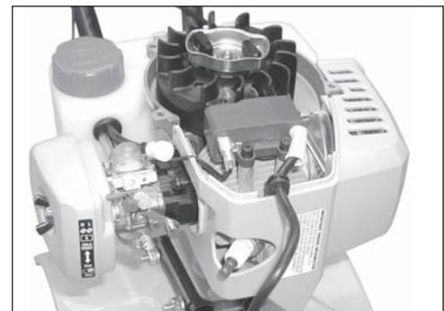
3. Remove bottom left (A) and bottom right (B) screws from cylinder cover.
