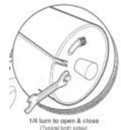
Lower the drum cover and return the sander to its upright position resting on the rear of the chassis.
