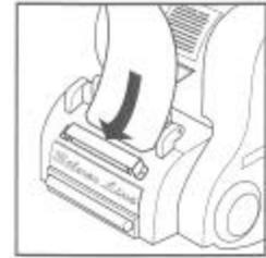
Tilt the SL-8 back onto the handle and lift the drum cover for easy installation
